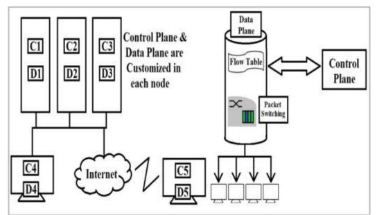
Figure 1 Traditional Network Vs Software Defined Network
