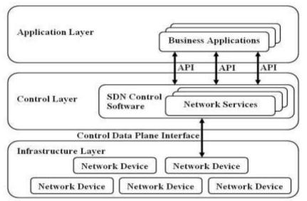
Figure 2 Structural Design of Software Defined Network
